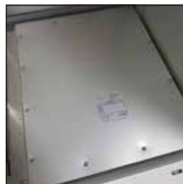
A4. Remove underlying caps by releasing their screws
